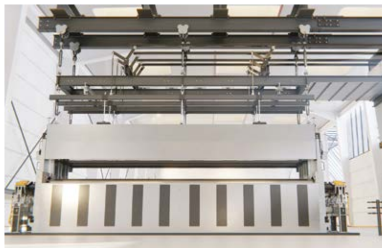
The dross box' housing has a stainless steel lining that is insulated and gas-tight.
