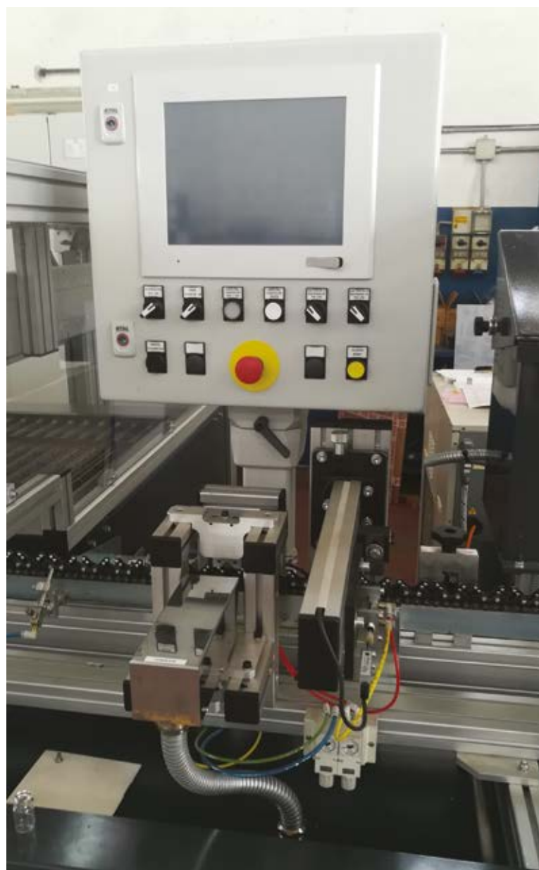
Complete station for dimensional inspection with dedicated control panel.
