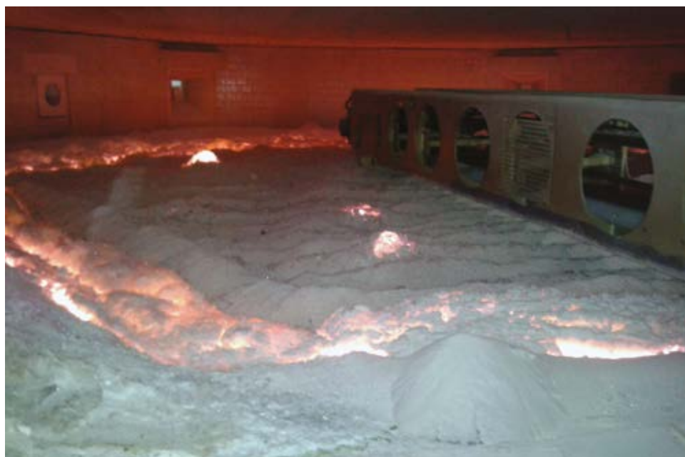
Cold batch on top of melt in full electric furnace.
