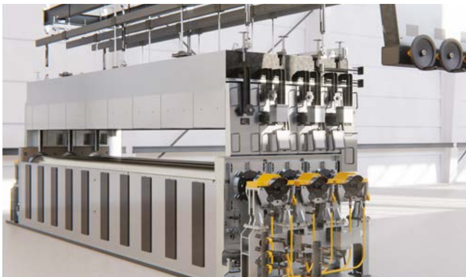
Grenzebach's new dross box ensures improved glass quality through a more homogeneous distribution of temperature across the entire width of the glass.
